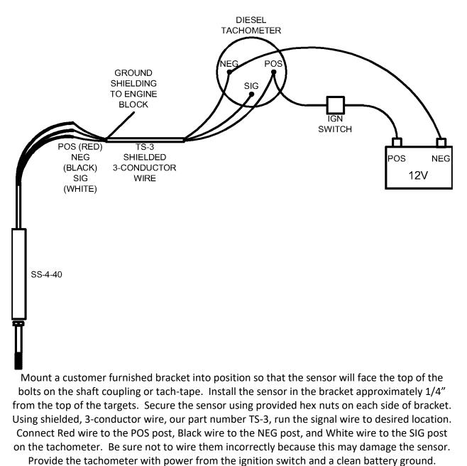
CAUTION – Damage due to incorrect wiring or contact with targets voids the warranty. NOTE: Ground the cable shield at the engine side of the signal wire only.
