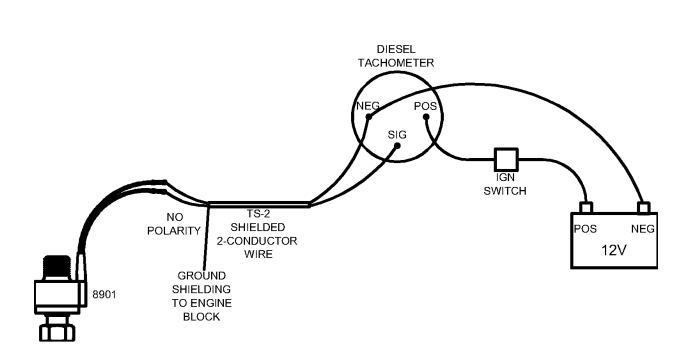
Verify that you have the correct size/style pin for the engine, and thread the unit onto the tachometer drive on the engine. Using shielded, 2-conductor wire, our part number TS-2, run the signal wire to the desired location. There is no polarity between the 2 wires, connect one to the SIG post and one to the NEG post on the tachometer. Provide the tachometer with power from the ignition switch and a clean battery ground. NOTE: Ground the cable shield at the engine side of the signal wire only.
