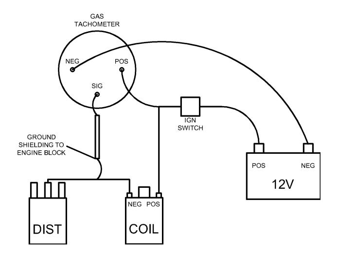
To install a tachometer on a Gas engine with a conventional ignition, provide power to the tachometer from the ignition switch and the battery ground. Using shielded wire, connect the negative side of the coil to the SIG post on the tachometer.
