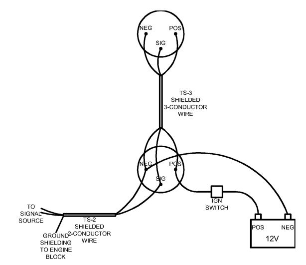
Follow the instructions for the correct signal generator while connecting to the first tachometer. Using shielded, 3-conductor wire, our part number TS-3, run the wiring to the second location. Connect the SIG to the SIG post, the POS to the POS post, and NEG to the NEG post on the second tachometer.
