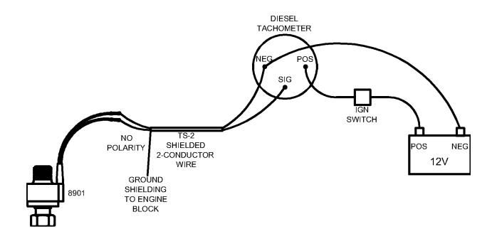
Verify that you have the correct size/style pin for the engine, and thread the unit onto the tachometer drive on the engine. Using shielded, 2-conductor wire, our part number TS-2, run the signal wire to the desired location. There is no polarity between the 2 wires, connect one to the SIG post and one to the NEG post on the tachometer. Provide the tachometer with power from the ignition switch and a clean battery ground.
