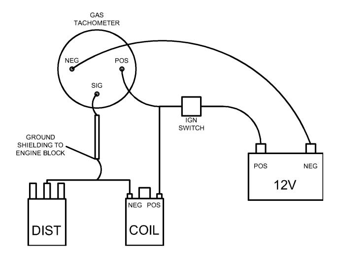
To install a tachometer on a Gas engine with a conventional ignition, provide power to the tachometer from the ignition switch and the battery ground. Using shielded wire, connect the negative side of the coil to the SIG post on the tachometer.
