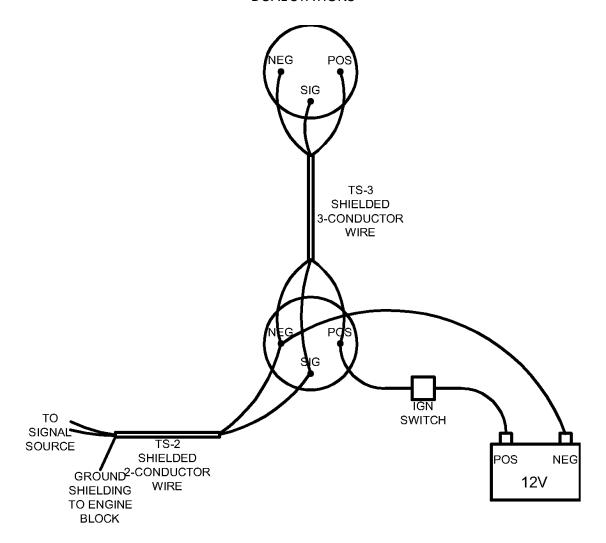
Follow the instructions for the correct signal generator while connecting to the first tachometer. Using shielded, 3-conductor wire, our part number TS-3, run the wiring to the second location. Connect the SIG to the SIG post, the POS to the POS post, and NEG to the NEG post on the second tachometer.
