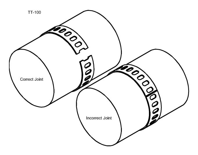
Calculate the length of tach-tape. Clean the area that the tape will be adhering to. Wrap the tape around the shaft and make sure that the joint completes a full oval. In higher speed applications, reinforce the tach-tape with a fiberglass-plastic tape. Wrapping the in the opposite direction that the shaft will spin to keep the trailing end from peeling. Never allow the tach-tape to come into contact with a high AC or DC magnetic field because this will damage the tach-tape.
