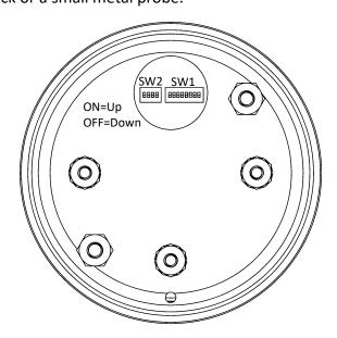
If you have are experiencing erratic RPM readings on a gas or outboard engine, the settings shown at the back of the manual can be applied to act as a signal filter and should stabilize the RPM reading.
